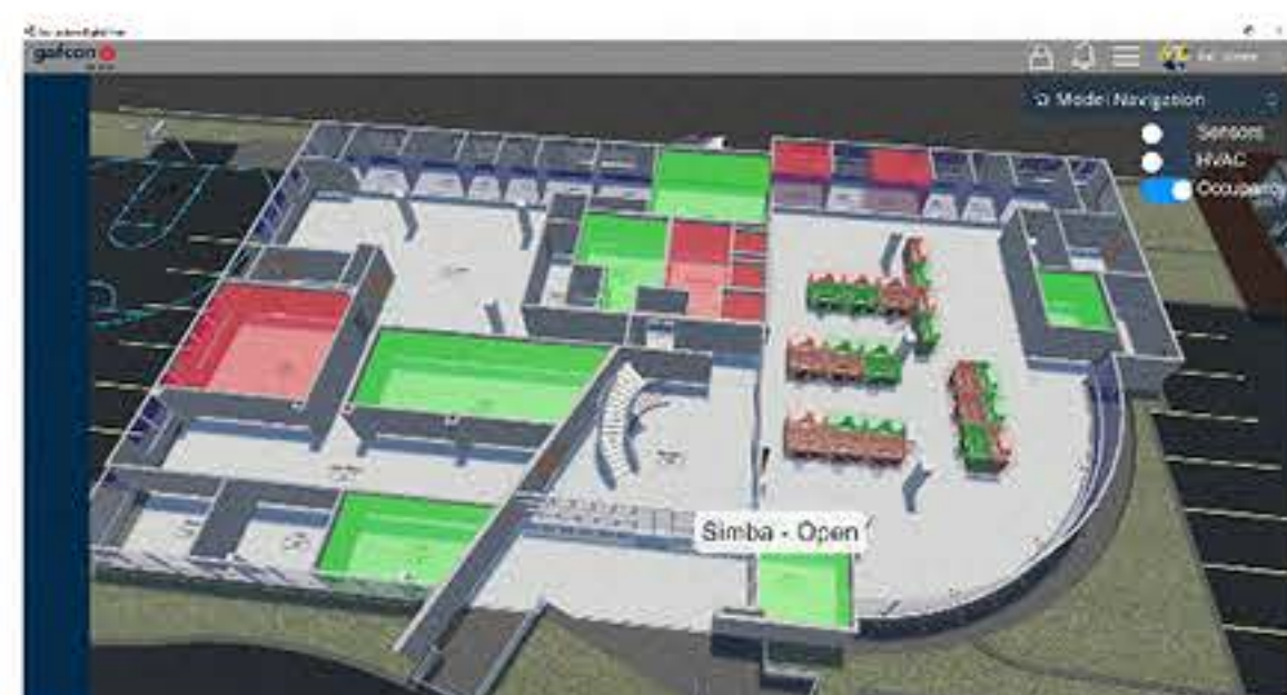
Gafcon Digital's home office modeled virtually, displaying work stations and rooms in different colors to indicate which ones are vacant and those that are being used. Illustration courtesy of Gafcon Digital
